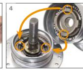
Check to make sure that the slide spring is While turning the hubshell left and right, Align the notches of the brake arm unit with the serrations of the brake shoe unit. Place the brake arm unit.
