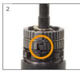
correctly positioned in the brake shoe unit. move it carefully downwards to place it.
