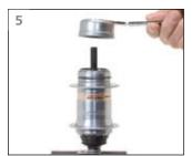
Remove the brake arm unit
