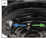
If the markings are aligned, the cable is correctly adjusted. After shifting down from 11 to 6, reconfirm the setting.
