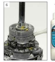
Reassemble the brake shoe and grease it with NEXUS grease (code number: Y-04120800).
