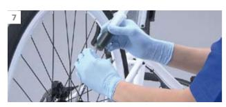
Carefully remove the syringe and tube containing the old oil.
