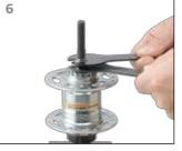
Assemble the left-hand cone and lock nut. Always adjust the hub so that the shell can be turned smoothly without any play after tightening.
