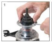
Hold the two flat surfaces of the hub axle in a vice. **Note:** Do not damage the threads of the axle. Carefully remove the right-hand dust cap.
