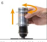
While turning the hubshell left and right. move it upwards to remove it. Do not use any force!
