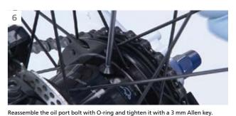
Tightening torque: 2-3 Nm.
