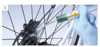
To reduce the pressure inside the hub, periodically pull the piston back a little.
