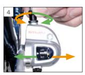
By turning the cable adjustment bolt, the setting can be changed. After shifting up from 1 to 2, reconfirm the setting.
