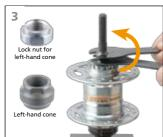
Turn the hub around and remove the lefthand lock nut and cone.
