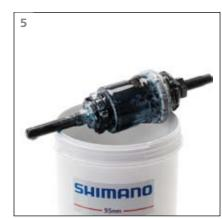
Let the excess oil drain off for approximately 60 seconds
