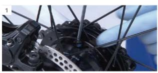
With the oil port in the upper position, remove the oil port bolt with O-ring using a 3 mm Allen key
