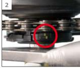
Check the alignment of the markings in the window of the cassette joint.
