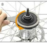
Turn the hub around and attach the right- On ALFINE 8-Speed hubs, use the special tool TL-AF10 to tighten the dust cap. Note the direction!
