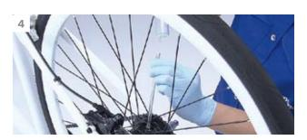
Once all the oil has been pushed out of the syringe, detach it from the tube to let the remaining oil in the tube flow into the hub.
