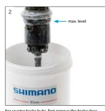
For coaster brake hubs, first remove the brake shoe unit! Immerse the internal unit into the oil from the left side. Immerse until the oil reaches up to the top of the
