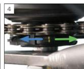
If the markings are aligned, the cable is correctly adjusted. After shifting up from 1 to 4, reconfirm the setting.
