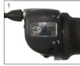
Shift up from gear 1 to gear 4.
