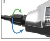
If the alignment is not correct, adjust it with the cable adjustment bolt on the
