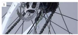
Wait 5 minutes until the oil has settled. Pull the syringe's piston slowly to drain all the old oil from the hub.
