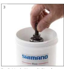
Keep the internal unit immersed in this way for roximately 90 seconds.
