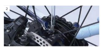
Attach the bleed nipple with O-ring and tube and tighten it using a 10 mm spanner. Tightening torque: 1-3 Nm.
