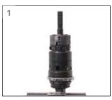
axle in a vice. Note: Do not damage the threads of the axle
