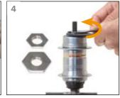
For coaster brake hubs, remove the 2 left-hand lock nuts to remove the brake
