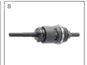
Now the internal unit can be used for the oil maintenance procedure as described on page 05.
