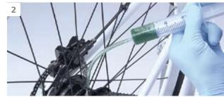
Assemble the bleed nipple with tube and attach the syringe. Push the piston slowly to inject the new oil into the hub.
