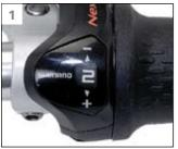
Shift up from gear 1 to gear 2.
