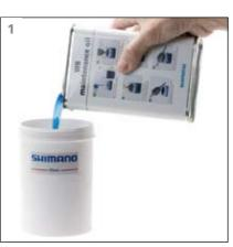
Fill the dipping vessel with WB oil.
