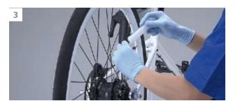
With the oil port still in the upper position, attach the syringe with its piston fully pushed in.
