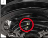
Check the alignment of the markings on the cassette joint.
