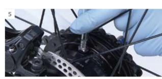
Remove the bleed nipple with O-ring and the tube.
