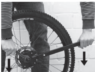
Illustration 5: Tightening the rear sprocket with the POM-Sprocket-Key and using the Open-end wrench SW24 to hold the Rohloff Sprocket tool in place.
