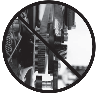
Illustration 4: Incorrect alignment of the belt
