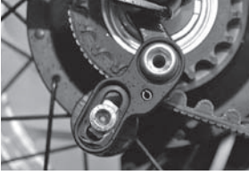
Illustration 3: Side view of the installed Snubber
