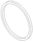
Shim ring for bottom bracket
