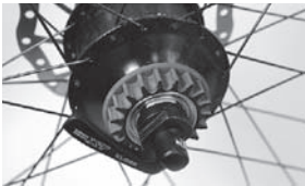
Illustration 2: Securing the Rohloff Sprocket tool with quick release skewer or axle nut
