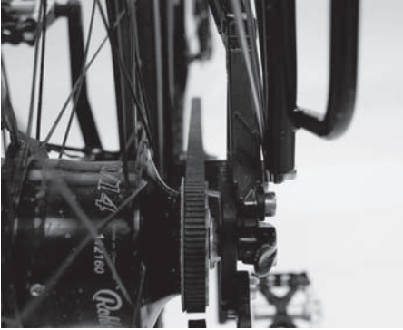
Illustration 3: Correct alignment of the belt
