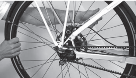
Illustration 3: Correct alignment of the belt
